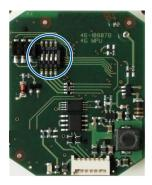
The address switch is used to set the hardware address:
