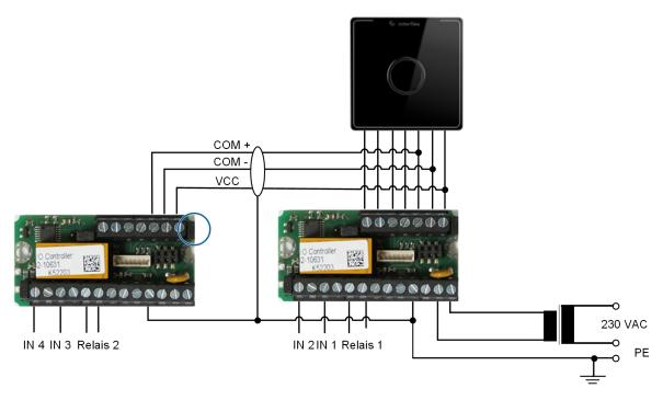
If more than two inputs or more than one relay are required, you can connect a second I/O controller board (accessory).
