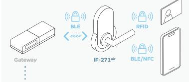
Investment protection by means of upgrade: Opendor card devices can be converted to Opendor air at any time.
